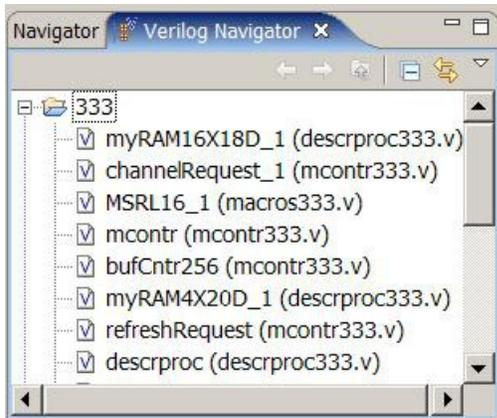
Non-VDT projects are shown as a list of files and directories, exactly as they are in the Navigator window. Moreover, there is a mode of the Verilog Navigator window to show VDT projects as files and directories, too. To switch the mode, press the white arrow at the right of the local tools panel of the Verilog Navigator window and choose a mode in the **Show** item:
