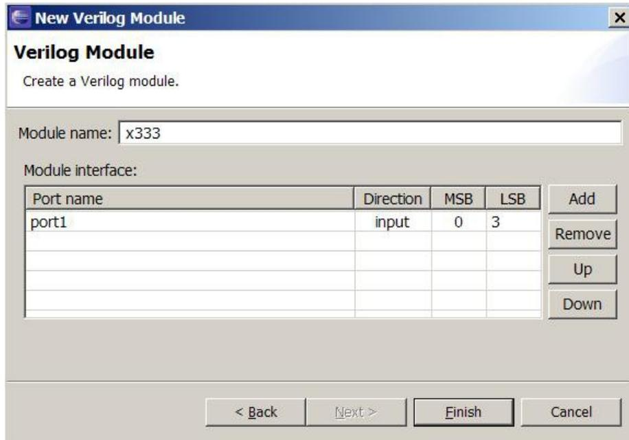
6) When the interface specification is over, press the **Finish** button. In the chosen project directory a new file with the specified name will be created, and a module template with the specified interface will be inserted in it.
