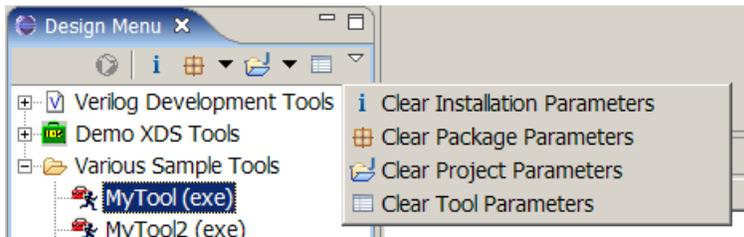
The Clear Package Parameters and Clear Project Parameters items discard saved values only for packages and projects available in the current Design Menu. The Clear Tool Parameters item discards saved values only for the selected tool.
