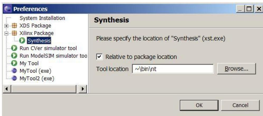
When a relative path is chosen, the package path, which is a prefix of the absolute path returned by "Browse", is automatically replaced by ~.
