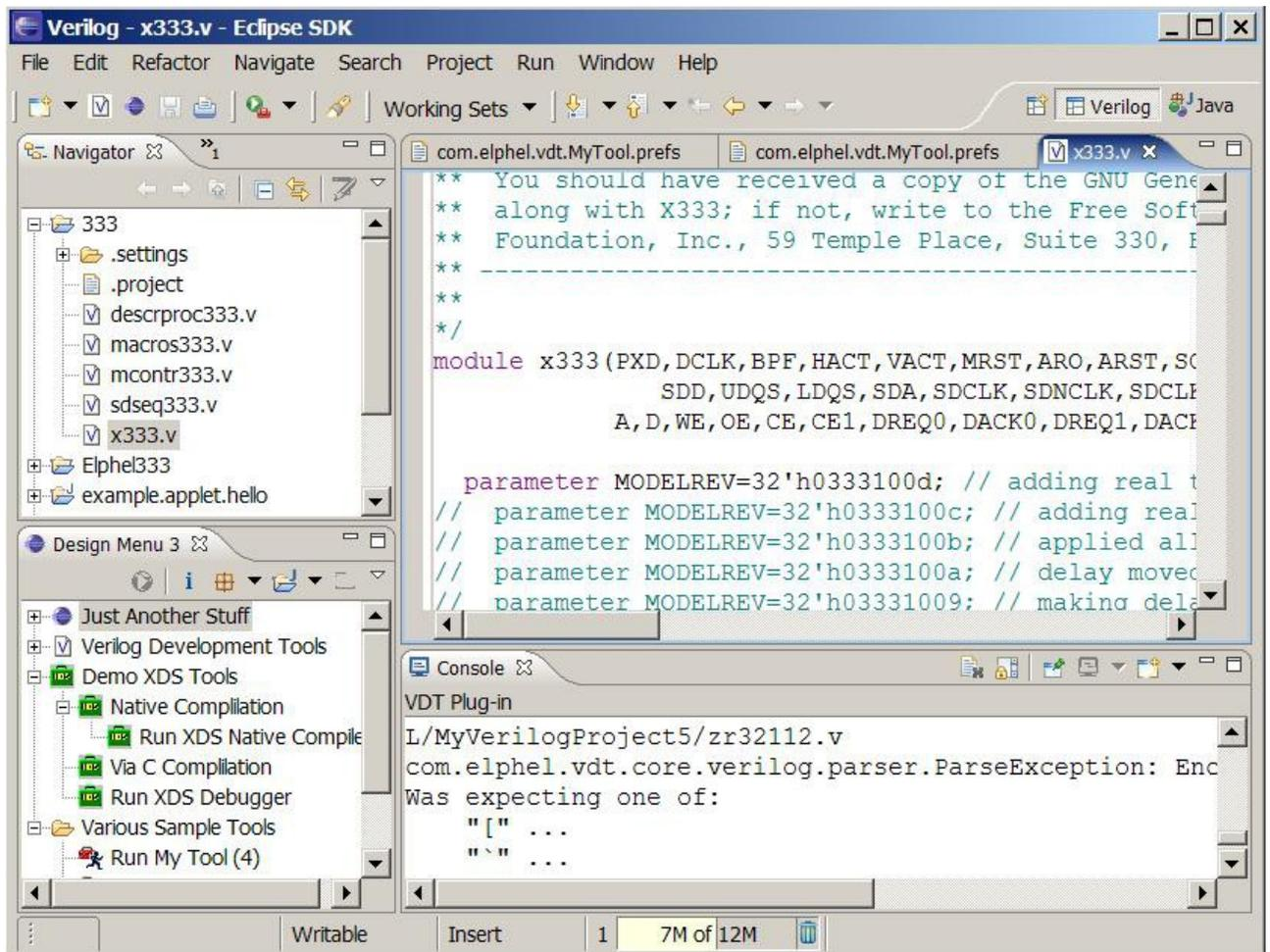
The central area of the Eclipse window is the text view window, where one or more files may be opened to edit. Syntax of texts may be highlighted according to their file types. E.g., files with extension `.v` are recognized as Verilog programs and highlighted according to Verilog syntax (if the Verilog editor plugin is installed).
